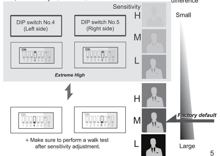
+ Make sure to perform a walk test after sensitivity adjustment.
